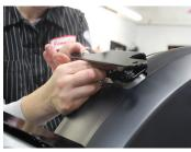
Install the rear seat bracket to the motorcycle frame using supplied hex bolts and washers finger tight
