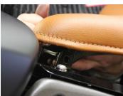
10. Set seat onto the rear bracket and align the front bracket so it slides in between the tabs on the seat pan
