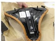
8. Install front seat bracket onto the bottom of the seat in the kit using 2 of the supplied carriage bolts, washers and lock nuts finger tight
