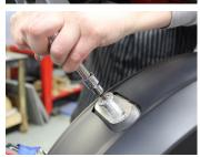
4. Remove the barb fitting on the fuel tank bracket plate and the rear mount post assembly
