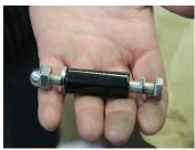
11. Install bushing in the vacant space inside the front mount bracket and install supplied long hex bolt with washers and acorn nut to secure
