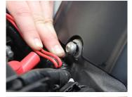
**6.** Install button head bolt with spacer into threaded hole at the rear of the seat area **TORQUE TO:** 6-8 ft-lbs
