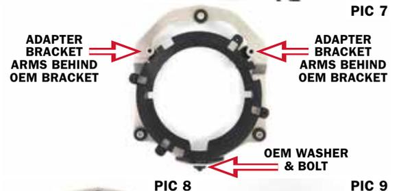
**STEP 7** Refer to PIC 7. Locate the OEM washer and screw that were removed from the bottom of the OEM bracket and carrier in Step 4. Place the washer onto the bolt, and insert through the bottom mounting holes of the bracket and adapter.
