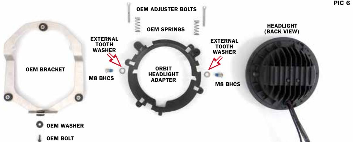
**STEP 6** Refer to PIC 7. Align the Orbit Headlight Adapter with the OEM bracket. The top two bracket arms of the Headlight Adapter should be placed under the bracket, and the bottom boss on the adapter should align and insert into the rubber grommet on the bottom of the OEM bracket.
