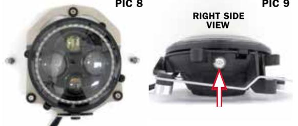
**STEP 9** Refer to PIC 8 and 9. Place an external tooth washer onto each of the 14mm screws. Fasten the headlight to the Orbit Headlight Adapter, from the left and right side. Fully tighten hardware.
