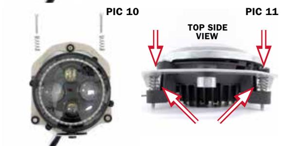
**STEP 11** Refer to PIC 11. Align the two bracket arms at the top of the Orbit Headlight Adapter with the OEM bracket. Place a spring in between the adapter bracket arms and the OEM bracket. From the top of the OEM bracket, insert the headlight adjuster bolts through the mounting holes of the OEM bracket, the springs, and bracket arms of the adapter. Lightly tighten the screw until brackets are fastened together.
