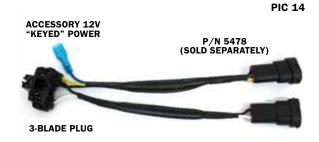
**STEP 10** FOR 14-UP H-D MODELS Refer to PIC 15. Connect the headlight's 3-blade connector to the connected adapter.
