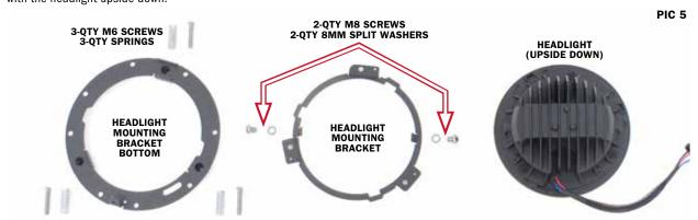
STEP 5 Refer to PIC 6 and 7. With the brackets of the Headlight Mount Bracket facing up, feed the wires of the headlight through the bracket and place it on top of the headlight.
