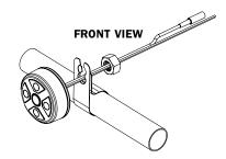
The unit can be clamp mounted using the included hardware.
