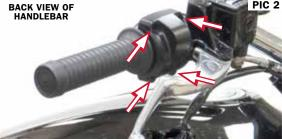
STEP 3 Refer to PIC 3. Note how the plastic throttle sleeve fits into the channel in the switch housing. Carefully slide the existing grip off of the handlebar.
