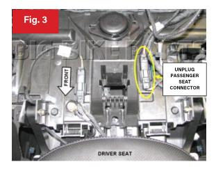
**5.** Disconnect the passenger seat wire harness as indicated in **FIG. 3**. Set the seat aside on a clean surface or towel.
