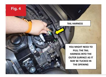
**6.** Locate the stock OEM tail harness location on the left side where the passenger seat is usually located. See **FIG. 4.**
