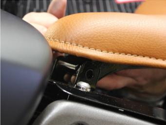
10. Set seat onto the rear bracket and align the front bracket so it slides in between the tabs on the seat pan
