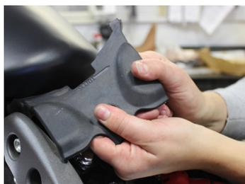
3. Remove the rubber flap over the fuel tank mount by pulling at an angle
