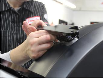
9. Install the rear seat bracket to the motorcycle frame using supplied hex bolts and washers finger tight
