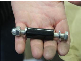
11. Install bushing in the vacant space inside the front mount bracket and install supplied long hex bolt with washers and acorn nut to secure
