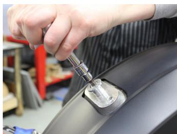
4. Remove the barb fitting on the fuel tank bracket plate and the rear mount post assembly
