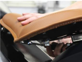
12. Install flat washer, lock washer and nut to each of the rear seat mount studs.
