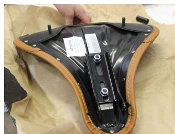
8. Install front seat bracket onto the bottom of the seat in the kit using 2 of the supplied carriage bolts, washers and lock nuts finger tight
