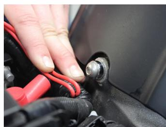
6. Install button head bolt with spacer into threaded hole at the rear of the seat area
