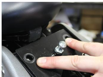
5. Remove the front two hex bolts on the fuel tank bracket plate
