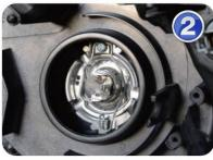
UNPLUG THE WIRE CONNECTOR AND REMOVE THE DUST BOOT.
