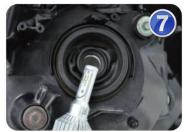
INSTALL THE NEW LED BULB THROUGH THE DUST BOOT AND INTO THE MOUNTING PLATE. ROTATE TO LOCK INTO PLACE.
