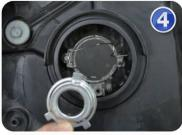
REMOVE THE MOUNTING PLATE FROM THE NEW LED BULB. INSTALL THE PLATE IN THE HOUSING.
