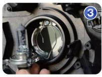
RELEASE WIRE SPRING CLIP AND REMOVE HEADLIGHT BULB
