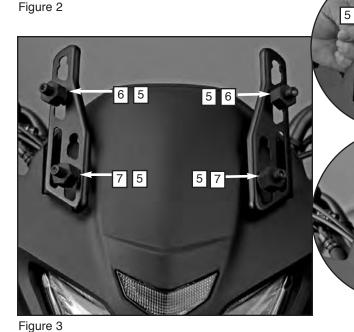
The bushings must be mounted in the lower mount position to avoid interference with mirror.
