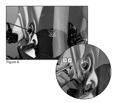
**4.** Tighten the Lower and Upper Bushings to 7ft-lbs. (9.5Nm). **(Box Wrench, Socket, Torque Wrench) Figure 4.**
