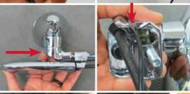
**STEP 22** Starting with the turn signal connector, feed the wires of the lights through the farthest back hole on the left side of the outer fairing. Align and insert the light assembly to the outer fairing.
