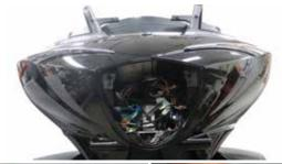
**STEP 17** Locate a Victory Driving Light, and one Pivot Mount from the Mounting Kit. With the beveled side of the Pivot Mount facing down towards the Driving Light, route the Driving Light's wire through the Pivot Mount. Be sure the wire is set inside the groove within the Pivot Mount. This will prevent pinching of the wire.
