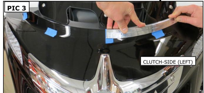
**STEP 5** Using the marks made in **STEP 3** align the Right Windshield Trim and press it into place for one minute; full bonding will occur after 24 hours. Repeat for the Left Trim.
